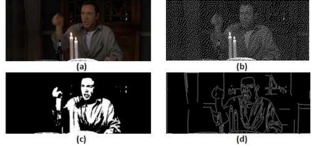
Figure 2. (a) original image. (b) created by dithering using [7], (c) created by thresholding the original image and (d) created by Canny edge operator respectively.
